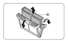
2. Open the outer filter and remove the inner filter (A).
