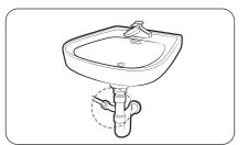
2. Connect the hose adapter directly to the drain pipe of the wash basin.
