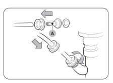
1. Assemble the hose connector (A), and attach it to the end of the accessory hose as shown.
