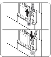
1. Remove the drain hose from hole (A), and insert it into part (B).
