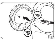
**12.** Tighten the 3 holder screws on the top. Then, tighten the 3 holder screws on the bottom.
