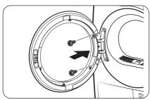
**10.** Insert the door hinge in the opposite position of the door frame, and then, tighten the 2 bolt screws.
