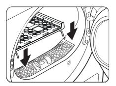
Position the drying rack in the drum, inserting the front lips of the rack into the holes of the door diaphragm.
