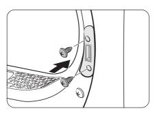
**9.** Insert the lever holder on the right frame, and then tighten the 2 holder screws.
