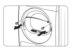
**5.** Remove the upper screw on the left of the door frame, and then insert it in the corresponding right hole of the door frame. Do not remove the lower bracket screws.
