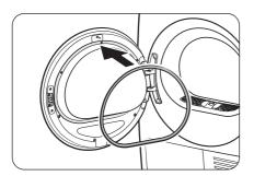
**13.** Attach the door packing to the door.
