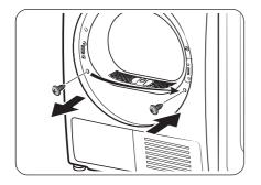
**8.** Remove the bottom screw on the left frame, and then insert it in the corresponding hole on the right frame.
