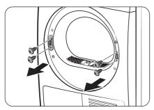
**6.** Remove the 2 bracket screws on the right frame, and then remove the 2 holder screws on the left frame.
