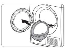
**11.** Insert the inner glass holder in the door cover that has been installed on the left frame.
