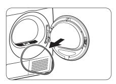
1. Remove the door packing from the door.
