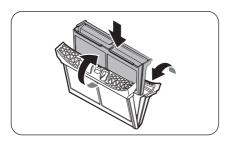
**5.** Put the inner filter into the outer filter, and then reinsert the lint filter into the original position.
