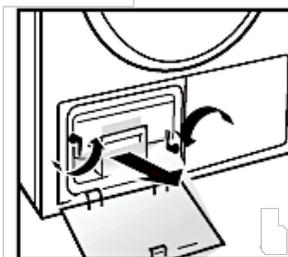
3. Clean the condenser under running water thoroughly. Drain the condenser thoroughly.
