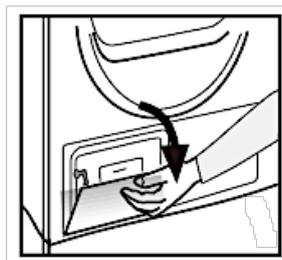
2. Unscrew the latches on both sides and pull out the condenser.
