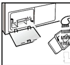
4. Reinsert the condenser into the opening properly.
