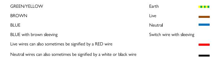
CLASS I Luminaires (Earthed) - Connect the brown wire from the luminaire to the supply live wire (red or brown). Connect the blue wire to the supply neutral wire (black or blue). Connect the green/yellow wire to the supply earth wire (green/yellow) or connect the supply earth to the luminaire earth terminal marked:
