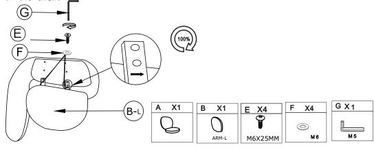
Assemble the Arm(R) to the bottomside of the seat with the 4pc. Bolts(E) and tighten them with the L-key(G). Make sure the arrow on the bottom of arm points to the frontside of the chair.
