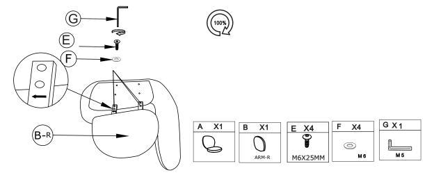
Assemble the frame to the bottomside of the seat with the 4pc. Bolts(D) and tighten them with the L-key(G). Make sure the arrow on the assembly plate points to the frontside of the chair.
