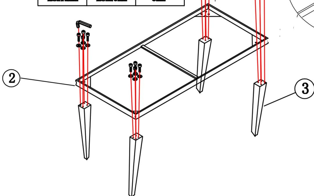
Note: Don't make screws tight until four legs are all connected with frame.
