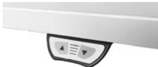
Press the 'down' button on the controls and hold it down. After 10 seconds the table will move to the lowest position and a small 'click' can be heard.
