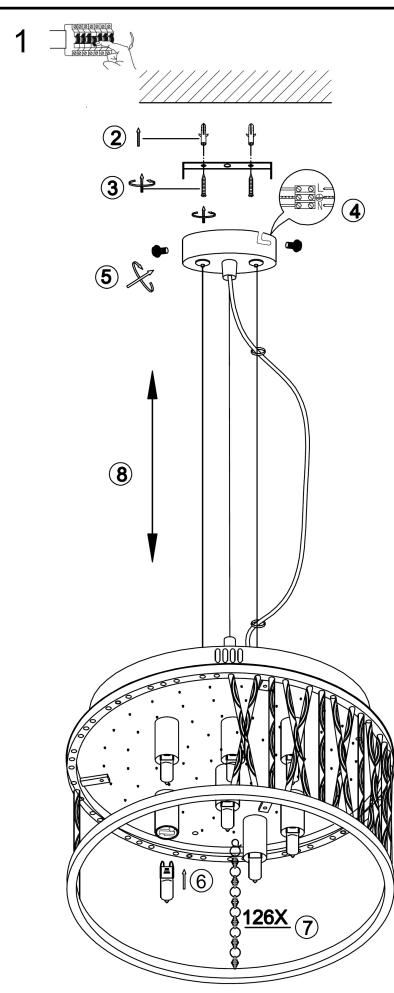
The 2 support wires attached to the fitting allow adjustment of the fitting, the height can either be reduced or increased.
