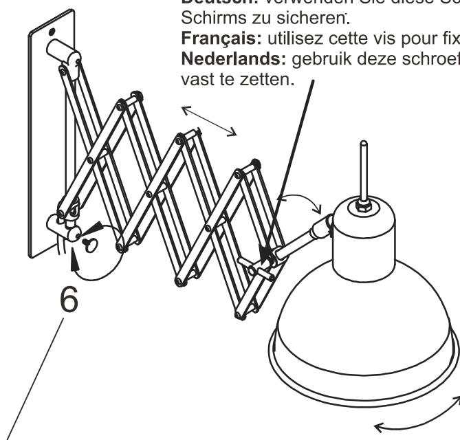
**English:** to reposition arm to left/right side, loose screw first and tighten again.
