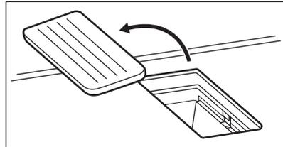
2. Take out the grease filter housing by grabbing the protruding handle.
