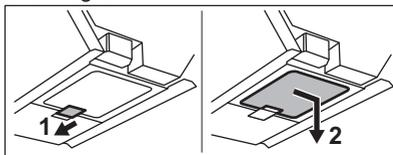
2. Move the drip tray vertically downwards. Be careful not to spill the water.
