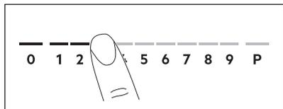
1. Press the desired heat setting on the control bar.
