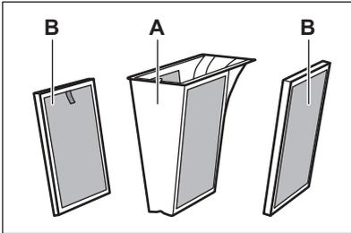
The grease filters **A** collect grease, oil, and food remains and prevent them from getting into the hood system. The long life carbon filters **B**, containing active carbon foam, neutralise smoke and cooking smells.
