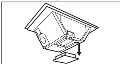
3. Dispose of the water and rinse the drip tray out. You can wash the tray manually (using soap and a soft cloth / sponge) or in a dishwasher (standard cycle).
