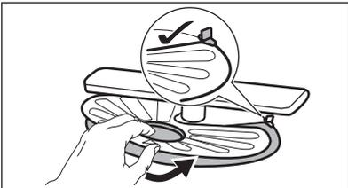
7. Reassemble the filters (B) and (C).
