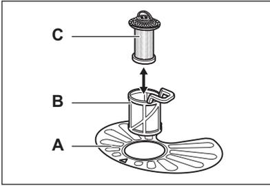
1. Turn the filter (B) counterclockwise and remove it.
