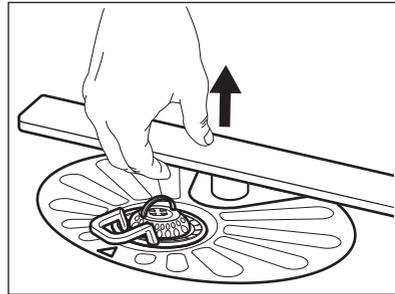
2. Wash the spray arm under running water. Use a thin pointed tool, e.g. a toothpick, to remove particles of soil from the holes. Run water through the holes to wash soil particles away from the inside.
