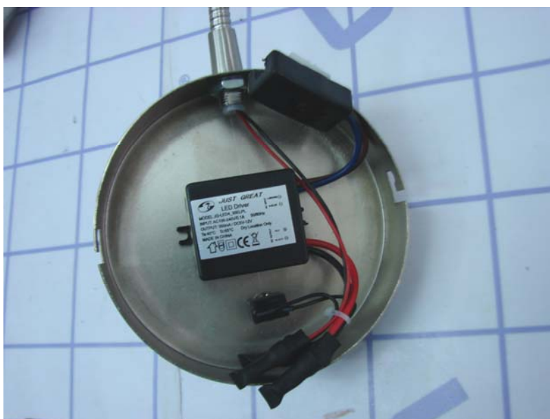
Figure 2 (internal view –LED driver)
