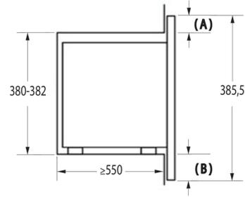
Installation of a microwave oven and frame overhangs: \*All dimensions in mm
