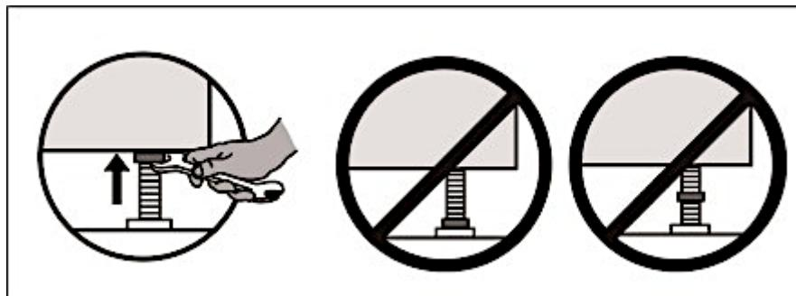
**NOTICE!** Do not turn the adjustable feet out further than **absolutely necessary**! The further the adjustable feet are turned out, the more the appliance may vibrate.
