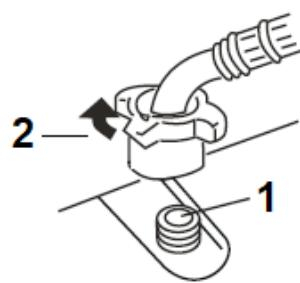
**NOTICE!** Do not overtighten the water inlet hose. Overtightening of the water inlet hose can damage the valves.
