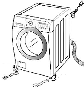
2. Turn the adjustable feet for horizontal alignment.
