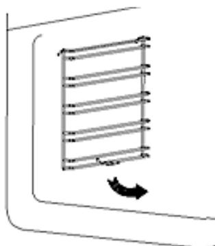
3. Unhook the side rack at the top and then pull it out **carefully** (s. fig. on the right, arrows).
