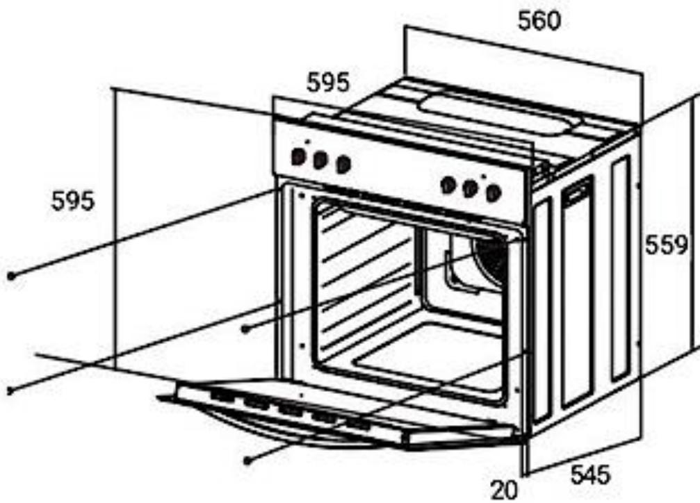
FIG. 2: DIMENSIONS OF THE INSTALLATION OPENING
