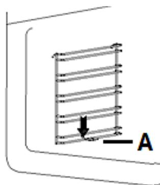
2. Swivel the side rack inwards at an angle of approx. **45 degrees** (s. fig. on the right, arrow).
