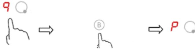
3. The maximum operating period of the BOOST FUNCTION is **5 minutes**, then the relevant cooking zone will operate in the previous setting. The display of the power level indicator changes from "P" to level. "9".
