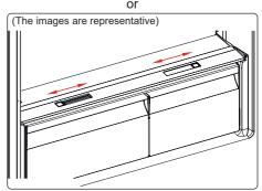
If the crisper is full, the fresh dial located in front of the crisper should be opened. This allows the air in the crisper and the humidity rate to be controlled, to increase the life of food within.
