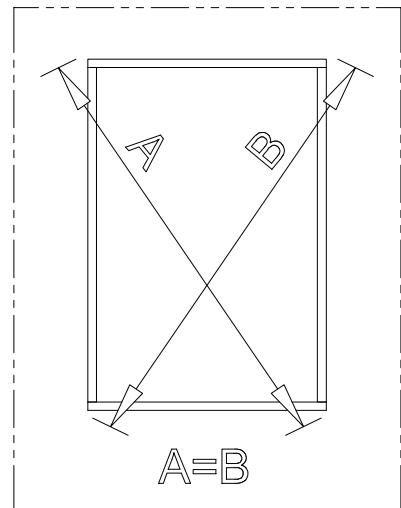
Regulate carefully before fastening to the wall
