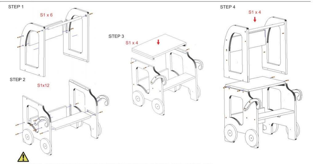
Ensure all screws and hardware are tightened and locked into place before use. Use only on a firm ground which is horizontal, level and dry.
