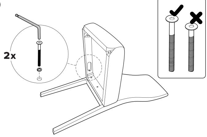
Fully engage all bolts halfway, engage U-Washer (Step 4). Finally, fully tighten using provided Allen Key.
