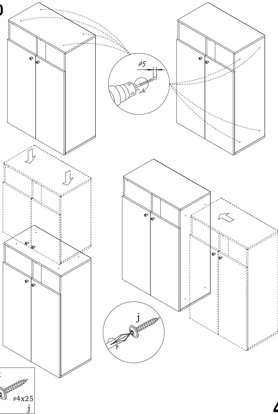
Diagram showing a self-tapping screw with the text "4x" above it and the part number "j" below it.
