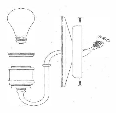
Secure the mounting plate to the wall with the two mounting plate screws.
