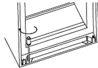
9. Fix the top bracket on the cabinet using short screws.
