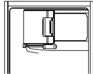
6. Move the bottom hinge pin from the right to the left side.
