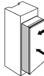
3. Fix one guide on the door of the appliance using short screws. Insert the slider into the guide. Then completely open and close the doors of the appliance and cabinet simultaneously to check, that the door of the cabinet opens and closes completely and smoothly.
