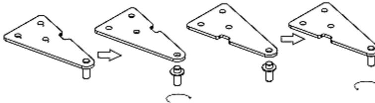
8. Insert the door. Then install the top hinge on the left side. Check that the door is adjusted properly and the door seals close properly before you finally tighten the screws of the top hinge.
