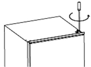
2. Unscrew the bottom hinge of the freezer compartment. Remove the door. Store the door at a place, where it cannot be scratched.
