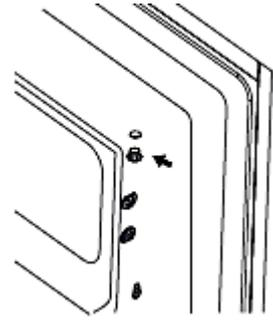
5. Rotate the freezer door and align the hinge side to the left side. Fix the door by holder.
