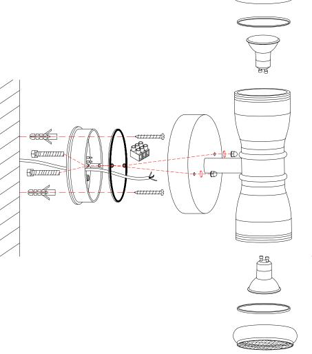
If this product is being installed outdoors, or a location where the product will be exposed to high levels of moisture, you should apply a silicone seal around the back-plate/canopy.
