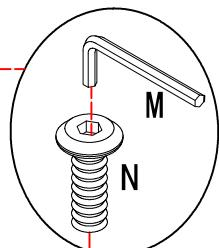
Do not tighten screws until all screws have been assembled!
