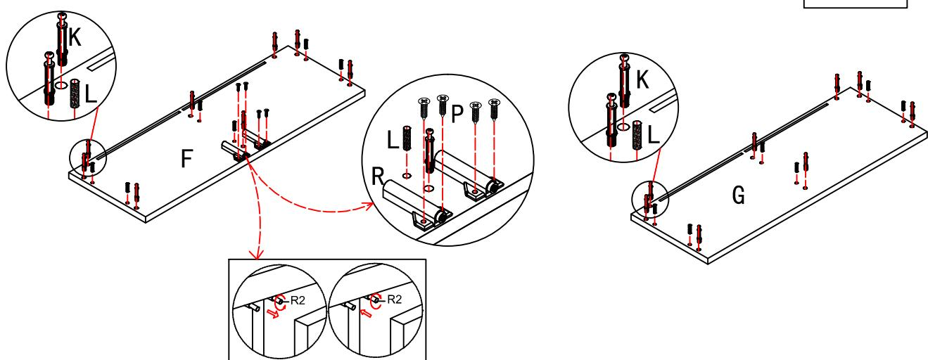
Do not tighten screws until all screws have been assembled!
