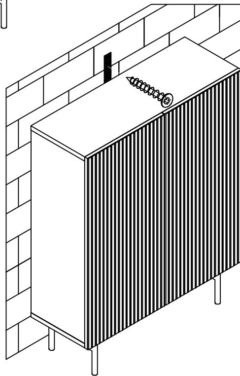
Do not tighten screws until all screws have been assembled!
