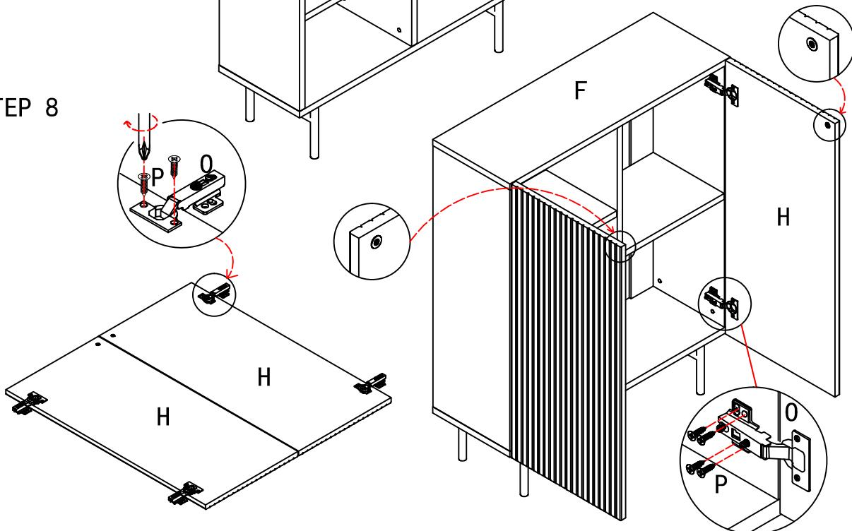
Do not tighten screws until all screws have been assembled!
