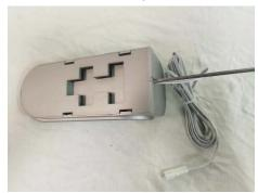
Step 2: Unscrew the light source plate using a screwdriver.
