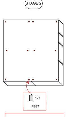
Turn the Base upside down and fix it on a flat surface. Then, mount the feet in the mounting package to the profile.
