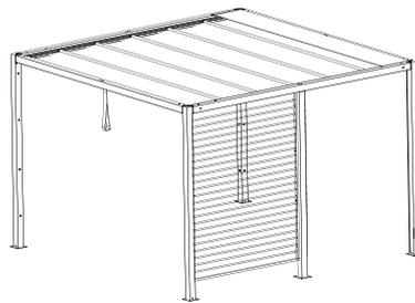
⊕ The SCREEN can be mounted on all 4 sides of the PERGOLA – left or right-justified.
