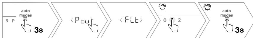
1. Immediately after connecting the appliance to the mains, touch the  $\equiv$  key for 3 seconds.
