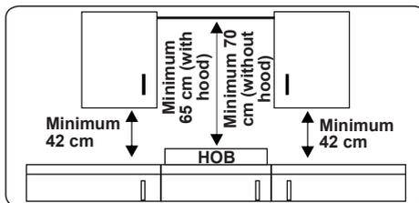
The appliance should not be installed directly above a dishwasher, fridge, freezer, washing machine or clothes dryer.
