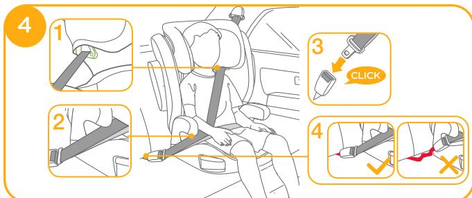
**GB** Installation using ISOFIX System and 3-point belt 1 - 4 or using 3-point belt only 4.
