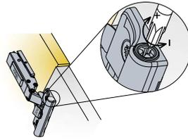
Damping is factory pre-set to the medium damping value. Turn towards '+' to increase and '-' to decrease the damping.
