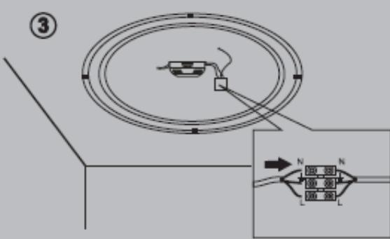
Open the quick connect terminal, take off screws and put the AC input line into it and fix screws back to finish connection.
