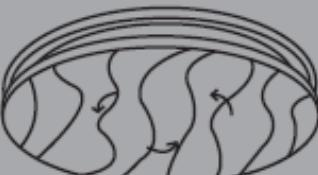
Put the PMMA cover back to the ceiling lamp and close the fixed button to complete the installation. Then connect with the main power for light on.
