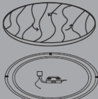
Open the fixed button and take the PMMA cover down.
