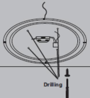
Drilling, push the lamp bottom to the ceiling and hold it by single hand, and then fix it by screws.
