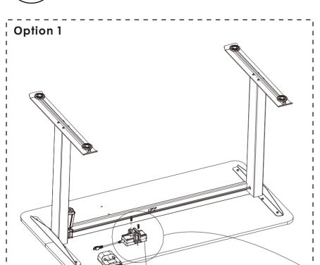
Note: Install the adapter and adapter box on the same side as the handset
