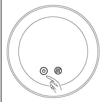
This is the switch for the LED light around the edge of the mirror. A short press switches the light on at it's first setting, Cool White 4000K. The switch will change from blue to white illumination, Another short press switches off the light and the switch reverts to blue illumination.
