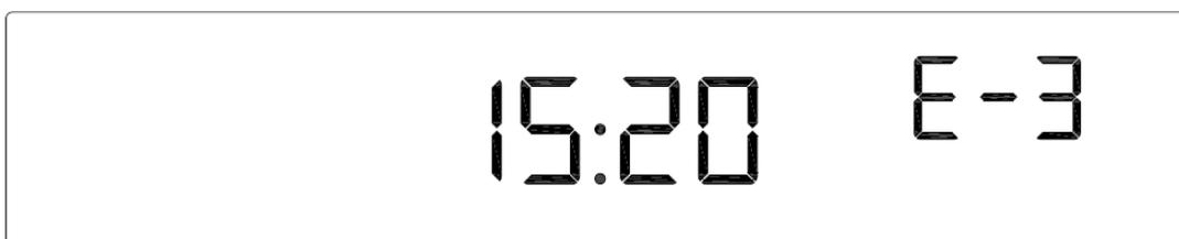
Pic 13: E-3 Door lock failure alarm diagram
