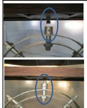
Match the iron bar (back of the wooden top) with the hole on the iron base, as shown in the picture. Secure the top with base using the bolt provided. Finger tighten the bolt. Check the angle of the top. Then fully tighten the bolt with the help of wrench provided.
