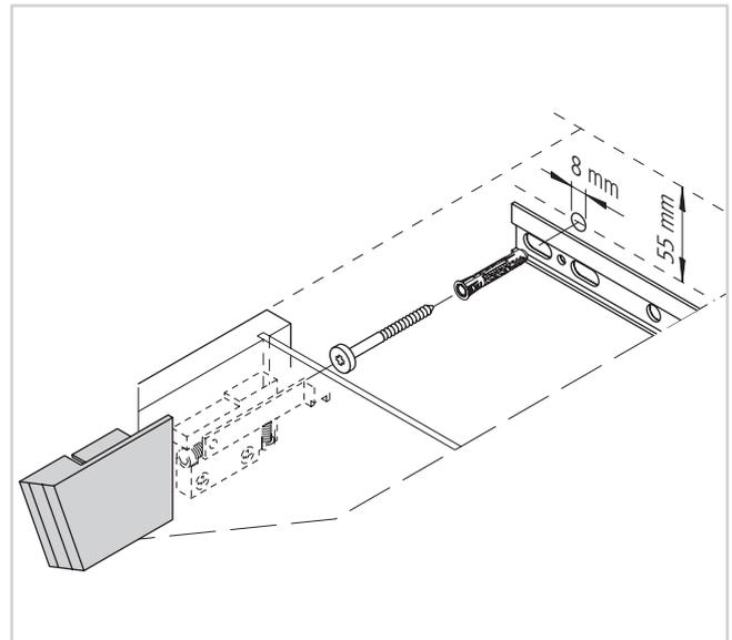
**DE** - Kippsicherung / **GB** - Anti-tipping device / **FR** - Anti-renversement / **NL** - Kantelbeveiliging / **ES** - Sistema de seguridad antivuelcos
