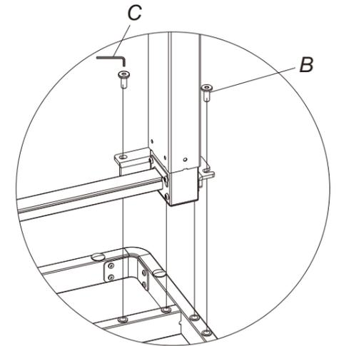
Use a hexagon allen key(C) and M8 screws to assemble the tabletop(1) and lifting columns(2).
