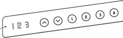
1. Touch the up/down button to adjust the height of the desk; the desktop runs to the lowest point and displays bot; the desktop runs to the highest point, displays top.
