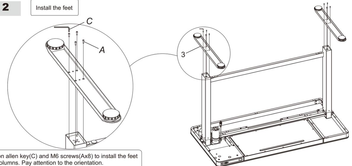
Use a hexagon allen key(C) and M6 screws(Ax8) to install the feet to the lifting columns. Pay attention to the orientation.
