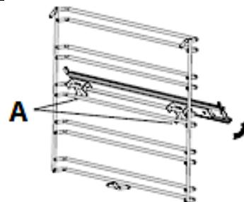
3. Lift the telescopic slide slightly so that you can remove it from the side rack without the slide hooks being jammed (s. fig. on the right, arrow).
