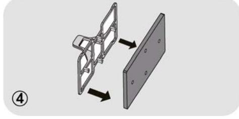
5. Wash the sponge by holding it under a running tap turning it so to remove any dust or fluff. Wring out the sponge and refit it carefully on the frame.
