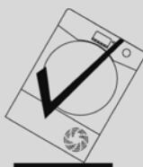
**If the product is in different side, wait at least 4 hours before switching on so that the oil can flow back into the compressor. Failure to do this could result in damage to the compressor.**
