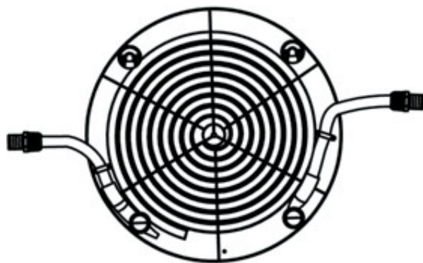
Assemble the 2 adaptors at the lower part of the solar heater
