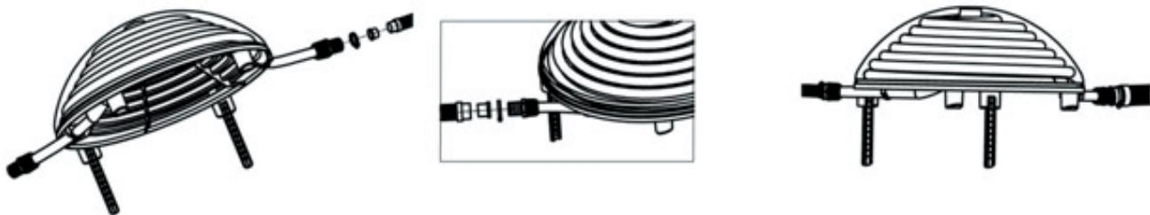
32 mm hosepipe adaptor: Connect this directly to the adaptor and fix it with the metallic clamps.
