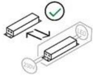
The diagram illustrates a separate operating device. It shows a small rectangular component on the left and a larger rectangular component on the right. A double-headed arrow connects them, indicating interchangeability. A green checkmark is positioned above the arrow. A small circular icon with 'LED' is visible on the larger component. |
