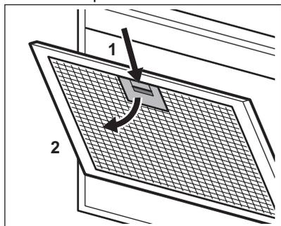
2. Slightly tilt the front of the filter downwards, then pull.
