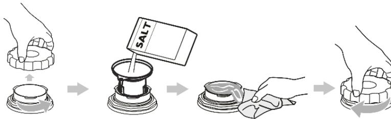
13. Remove the lower basket and unscrew the lid of the salt container.
