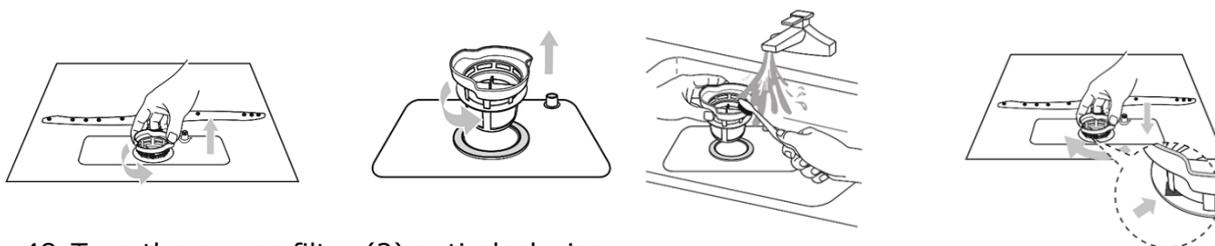
48. Turn the coarse filter (2) anti-clockwise and lift the filters upwards.
