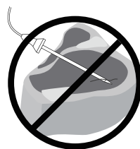
(Figure C) Incorrect placement of probe
