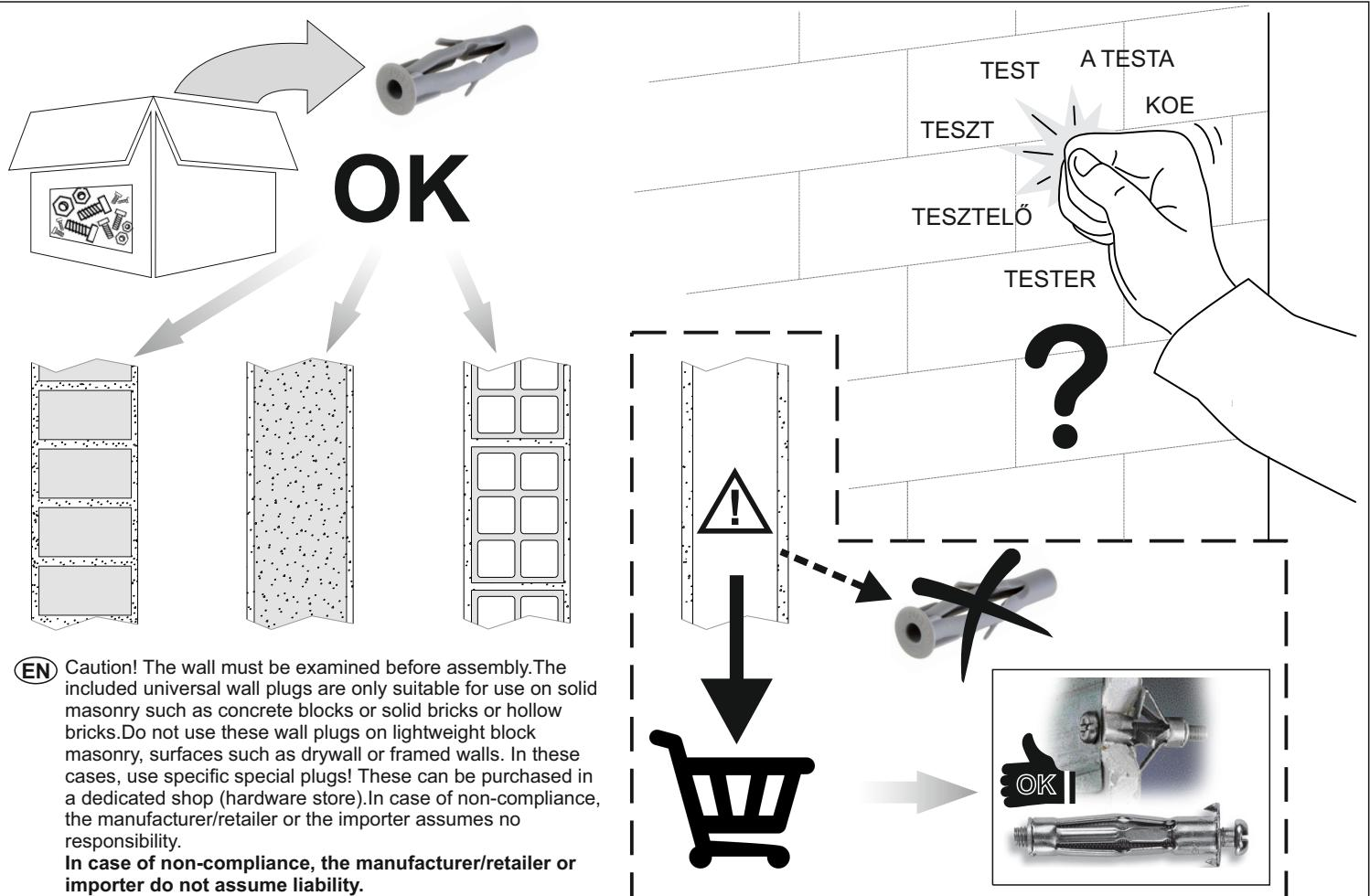
**(EN)** Caution! The wall must be examined before assembly. The included universal wall plugs are only suitable for use on solid masonry such as concrete blocks or solid bricks or hollow bricks. Do not use these wall plugs on lightweight block masonry, surfaces such as drywall or framed walls. In these cases, use specific special plugs! These can be purchased in a dedicated shop (hardware store). In case of non-compliance, the manufacturer/retailer or the importer assumes no responsibility.
