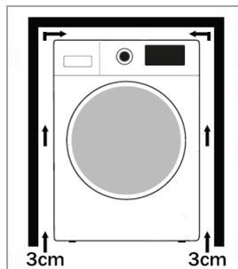
The appliance can only be positioned under a working plate if the minimum distances can be adhered as shown in the illustration.
