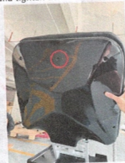
(The back panel of the seat package is fixed with a total of 5 70mm screws)
