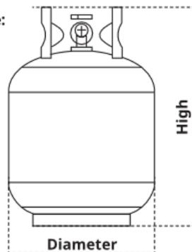
If your gas bottle does not fit into the bottle holder of the cabinet, it must be placed next to the grill at a distance of 60 cm from the side burner.
